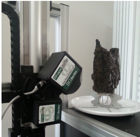
Fig. 5. Test sample positioned on top of a control object (see below test sample) and on a rotating stage to automate the 3D scan acquisition phase.
