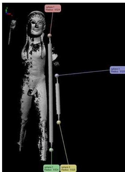
Fig. 11 – Accuracy verification: a) laser scanner intrinsic and extrinsic calibration b) stadia bars used to check the 3D model.
