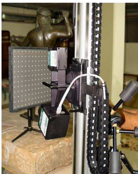
Fig. 11 – Accuracy verification: a) laser scanner intrinsic and extrinsic calibration b) stadia bars used to check the 3D model.
