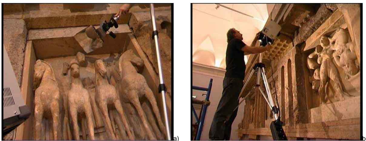
Fig. 4 - Practical considerations when using a 3D scanner: mirror used to reach hidden 3D surfaces.
