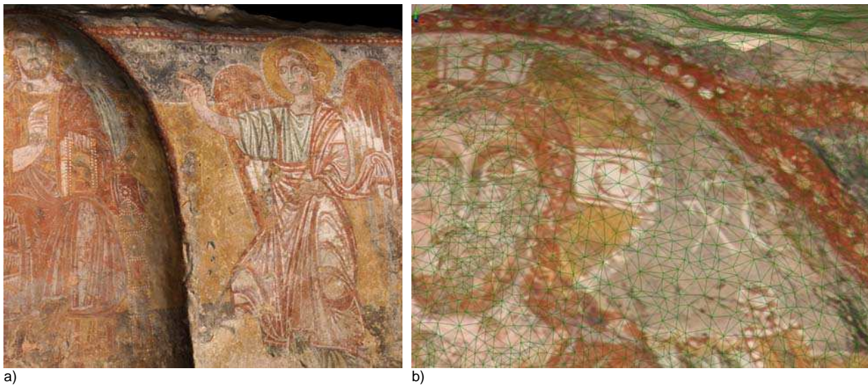
Fig. 1. Section showing Christ Pantocrator, a) coloured 3D model illuminated by one source of light, b) close-up showing the wire-mesh on which the colour was mapped ( the smallest triangle have sides of about 5 mm).
