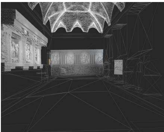
Fig. 6 - Virtualized Museum room: multi-resolution 3D model shown as a wire-mesh model.
