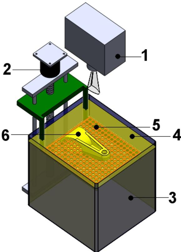
Fig. 8. Envisiontec Ultra Apparatus: 1. Light projector; 2. Motor – Z Axis Elevator Mover; 3. Vat; 4. Resin; 5. Platform; 6. Part in construction.
