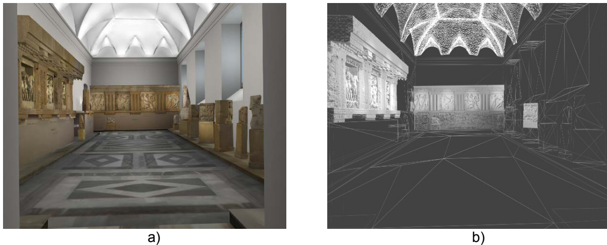
Figure 12. Virtualized Museum room, a) Rendering of the complete 3D model of the museum room dedicated to Selinunte, b) wire-mesh showing the multi-resolution 3D model.
