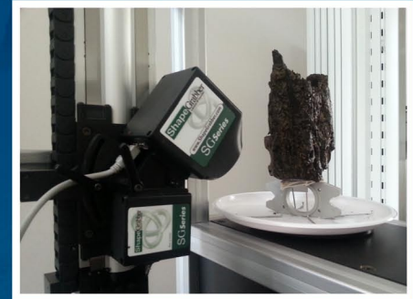
Fig. 5. Test sample positioned on top of a control object and on a rotating stage to automate the 3D scan acquisition phase.
