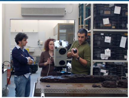
Fig. 3. Minolta VIVID 900 that was used for the 3D laser scans.
