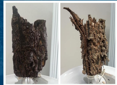
Fig. 6. The test sample. Its weight was 848 g when it was extracted from the water tank and drained of excess water. The test was concluded after eight days from the start day. The test sample was still wet and weighed now only 264 g.
