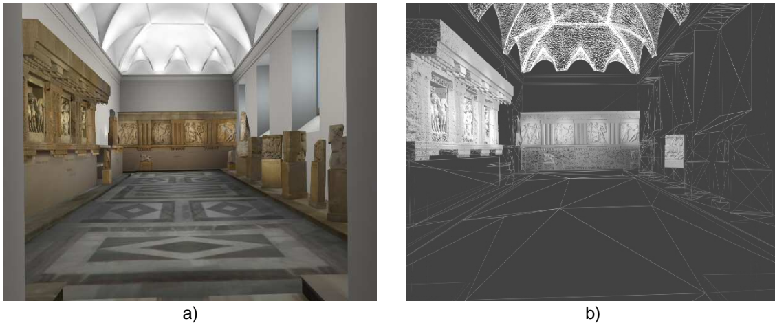
Figure 9. Model of the Museum room, a) Rendering of the complete 3D model of the museum room dedicated to Selinunte, b) wire-mesh showing the multi-resolution 3D model.
