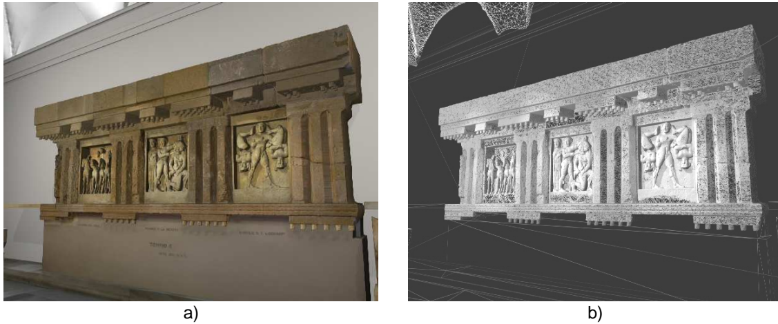
Figure 8. Three-dimensional model of a section of the frieze of Temple C of Selinunte, a) texture-mapped 3D model, b) wire-mesh of 3D model showing the levels of details.
