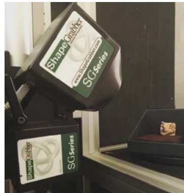
Fig. 1. Test sample positioned on top of the rotating stage. ShapeGrabber® AI300 + SG102.
